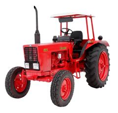
The tractor is designed for various agricultural operations with mounted, semi-mounted and trailed machines and implements, for transport operations.
